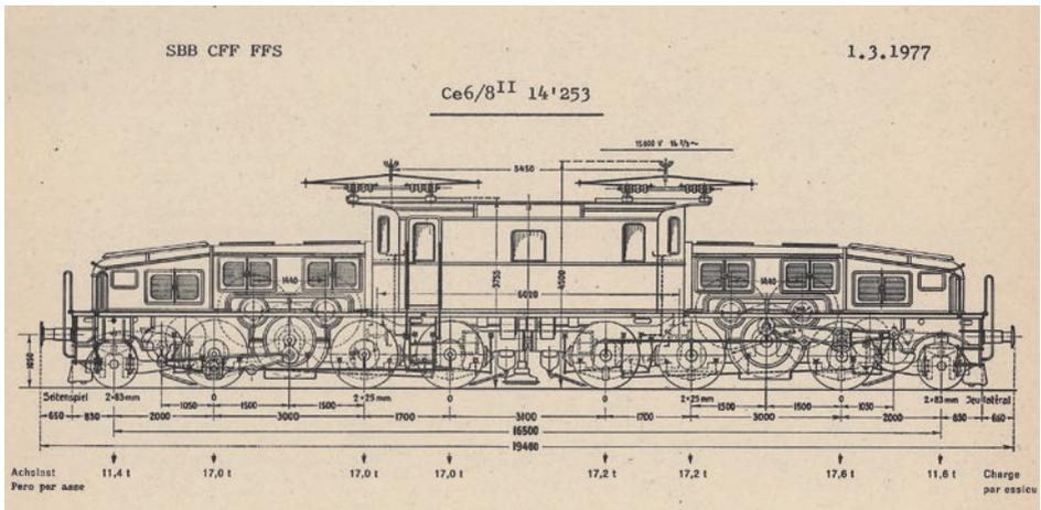
Figure 7: Sketch of the Ce 6/8 II with the main dimensions
