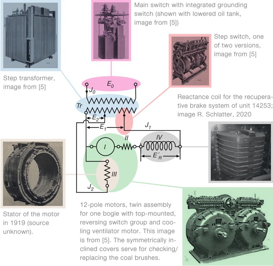
Figure 9: Ce 6/8 II components referring to the (simplified) electric scheme for electric recuperation, see [3]. The complete contemporary electric schemes are included in the publications [4] and [5].
