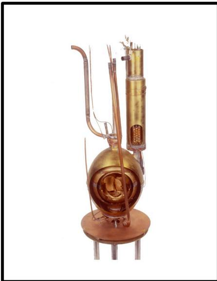
This calorimeter is the instrument used at the National Bureau of Standards, now known as National Institute of Standards and Technology (NIST), in the 1920s and 1930s to measure the heat of vaporization and related properties of steam at temperatures below 100 °C; these data still play a significant role in modern steam tables.
