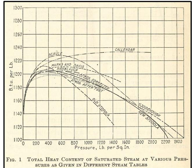
FIG. 1 TOTAL HEAT CONTENT OF SATURATED STEAM AT VARIOUS PRESSURES AS GIVEN IN DIFFERENT STEAM TABLES
