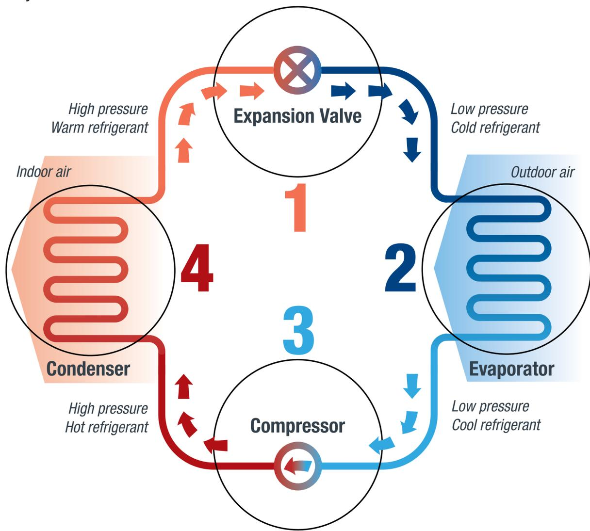
Heat pumps have a lot in common with air conditioners or refrigerators. They all have two sets of coils, with a motor to move refrigerant from one side to the other and back. The key is finding a refrigerant fluid with a low boiling point, so that it can absorb heat from low-temperature sources, such as the outside air on a frigidly cold day, as it makes a round trip through the system.
