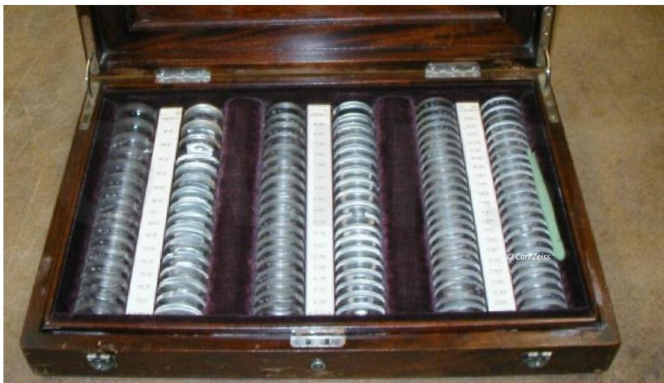
This is the AO primary true-power lens set calibrated by Edmund Tillyer when he worked at the National Bureau of standards prior to joining AO.
