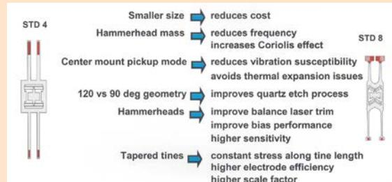
Figure 13 – Comparison between a STD 4 and STD 8 Hammerhead Quartz Tuning Fork (Source: BEI Technologies Inc.)
